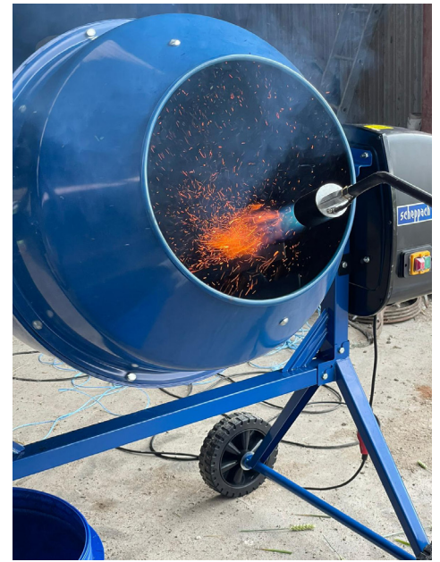
Above: Experimental processing of barley Freekeh using a rotating drum and gas torch.
