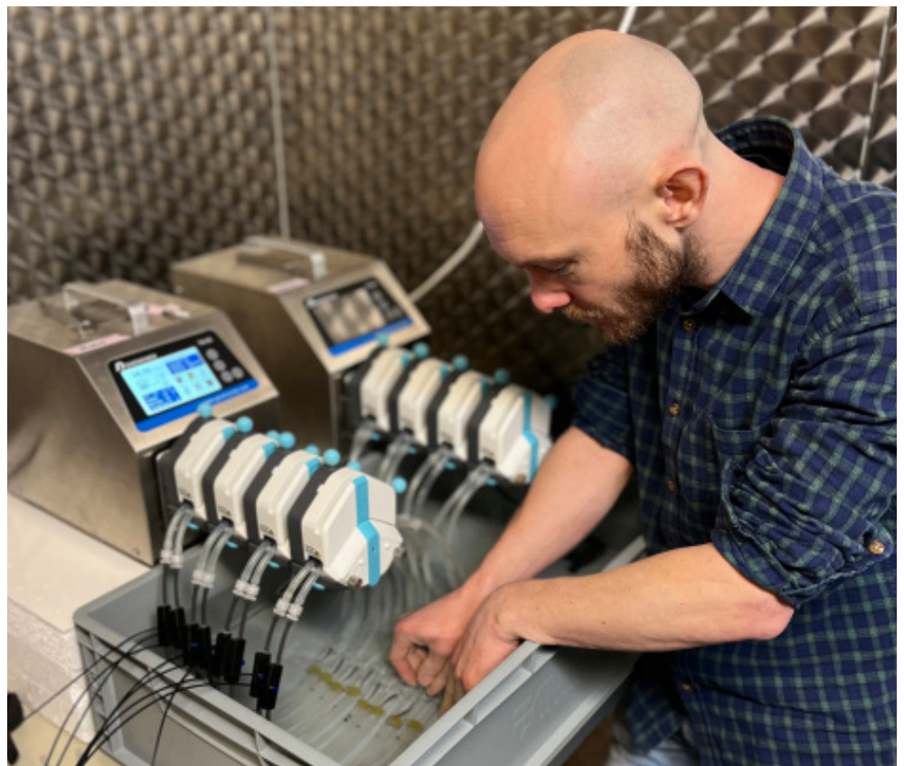
Above: Tommy is measuring oxygen uptake rates of small fish using so-called intermittent-flow respirometry to quantify the fish's metabolic rates.
